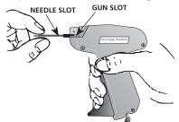
Turn needle lock toward the rear of the gun to lock needle in place.
