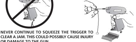
If a fastener can't be easily and safely removed from the needle simply replace the needle with a new one (as shown above).
