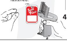
To remove fastener clip from gun — push fastener release button on top of gun toward rear of gun. Pull fastener clip straight up to remove from gun.
