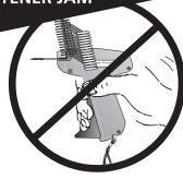
If a fastener jams: First release the trigger and remove the needle (as shown above). Then carefully remove the jammed fastener from the gun or needle.
