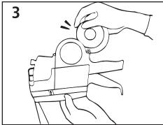
Load the label roll onto the LABEL-CASE.
