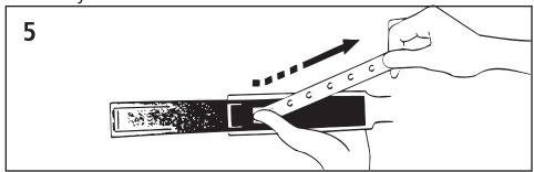
Fold back the label roll at the PRINT-PLATE-PIN while pressing the BASE-PLATE slowly.
