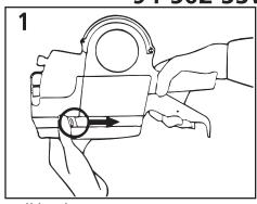
Pull back THE BASE-PLATE-OPEN-KEY as shown by arrow.
