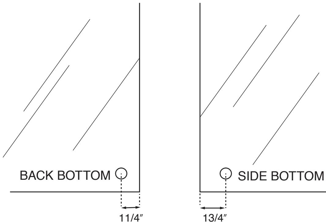
MEASURE THE GLASS SPACE BETWEEN EDGE OF GLASS AND CENTER OF HOLE. HOLE FURTHEST FROM EDGE GOES ON BOTTOM
