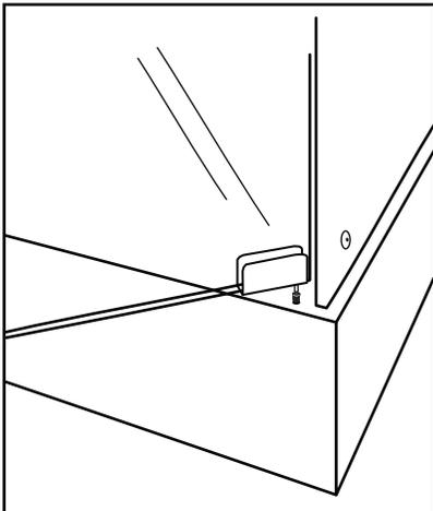
ATTACH **TOP RIGHT** OF FRONT DOOR (APPROXIMATELY 1/16" FROM EDGE OF GLASS) - **REPEAT** HINGE ASSEMBLY ON **BOTTOM**
