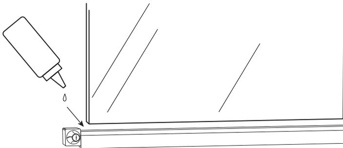
RUN BEAD OF ANY TYPE OF GLUE ON INSIDE (TOP) OF BOTTOM METAL SLEEVE. THEN TAP SLEEVES ON BOTTOM OF THE GLASS WITH A RUBBER Mallet.
