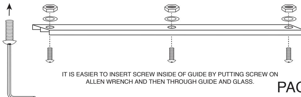
IT IS EASIER TO INSERT SCREW INSIDE OF GUIDE BY PUTTING SCREW ON ALLEN WRENCH AND THEN THROUGH GUIDE AND GLASS.
