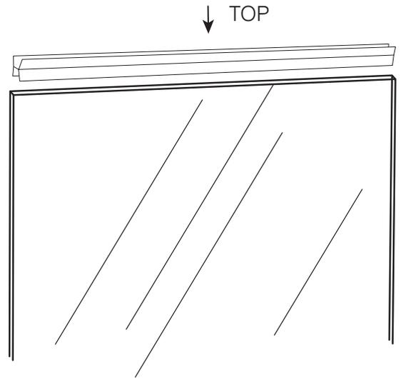
PLACE METAL SLEEVES (WITH LOCK TO THE LEFT) ON BOTTOM OF GLASS DOORS. TAP ON SLEEVES WITH RUBBER Mallet.
