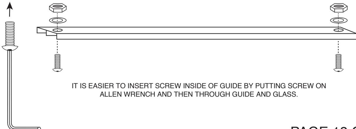
IT IS EASIER TO INSERT SCREW INSIDE OF GUIDE BY PUTTING SCREW ON ALLEN WRENCH AND THEN THROUGH GUIDE AND GLASS.
