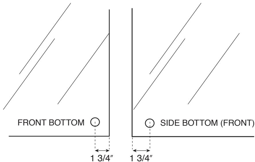
MEASURE THE GLASS SPACE BETWEEN EDGE OF GLASS AND CENTER OF HOLE.
