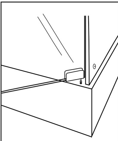
ATTACH **TOP RIGHT** OF FRONT DOOR (APPROXIMATELY 1/16" FROM EDGE OF GLASS) - **REPEAT** HINGE ASSEMBLY ON **BOTTOM**
