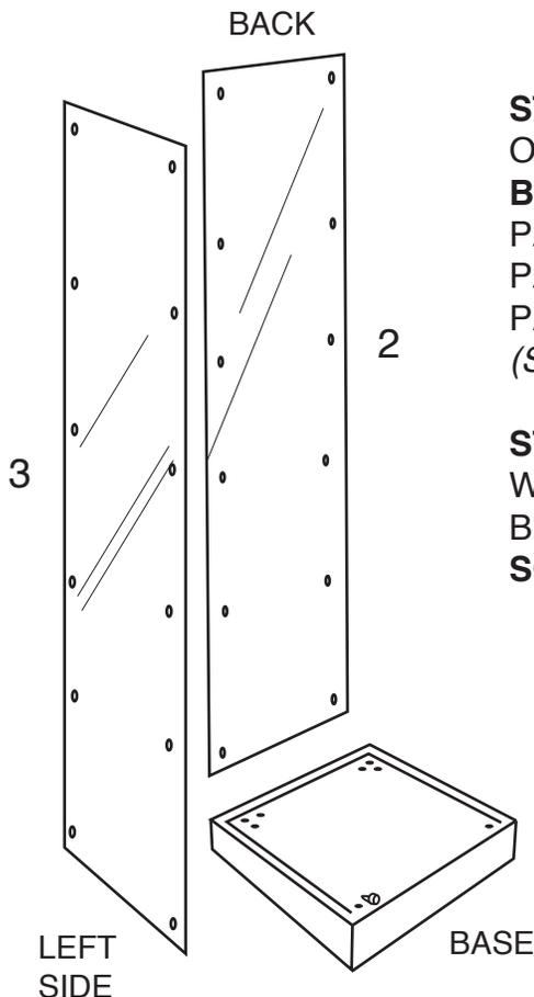
**STEP 2. PLACE BACK GLASS PANEL INTO BACK GROOVE OF CABINET BASE. MAKE SURE GLASS PRECISELY FITS BACK BASE GROOVE IN ORDER TO ACCOMADATE THE SIDE PANELS NEXT. MAKE CERTAIN ON BOTH BACK AND SIDE PANELS THAT YOU RECOGNIZE THE BOTTOM OF EACH PANEL CORRECTLY. (SEE DETAILS BELOW)**
