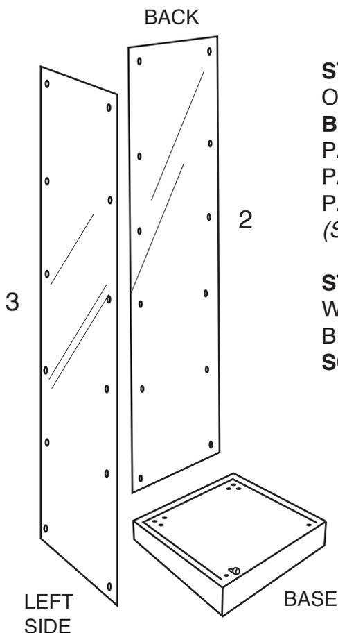
**STEP 2. PLACE BACK GLASS PANEL INTO BACK GROOVE OF CABINET BASE. MAKE SURE GLASS PRECISELY FITS BACK BASE GROOVE IN ORDER TO ACCOMADATE THE SIDE PANELS NEXT. MAKE CERTAIN ON BOTH BACK AND SIDE PANELS THAT YOU RECOGNIZE THE BOTTOM OF EACH PANEL CORRECTLY. (SEE DETAILS BELOW)**
