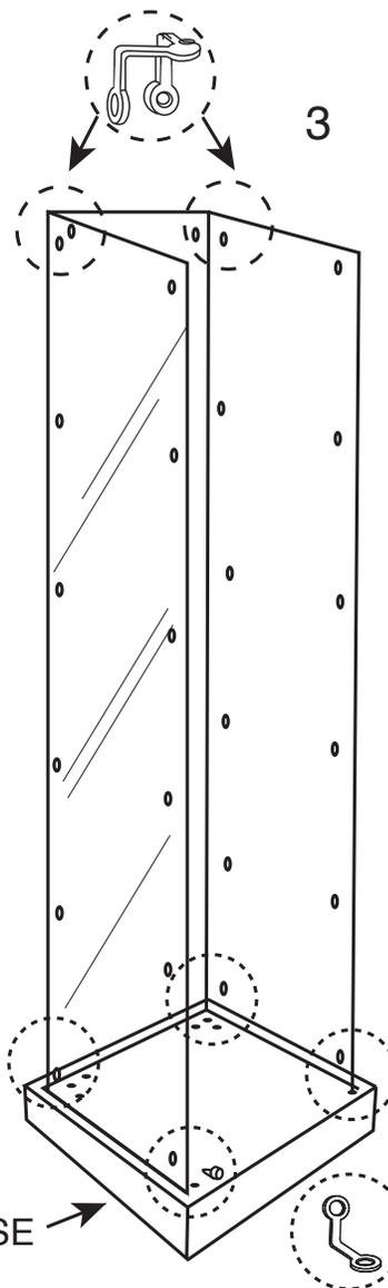
**STEP 5. PLACE TOP GLASS ONTO ASSEMBLY ALONG WITH ALUMINUM STABILIZING BAR ATTACHING ALLEN SCREW AND PLASTIC WASHERS AND L-BRACKETS.**
