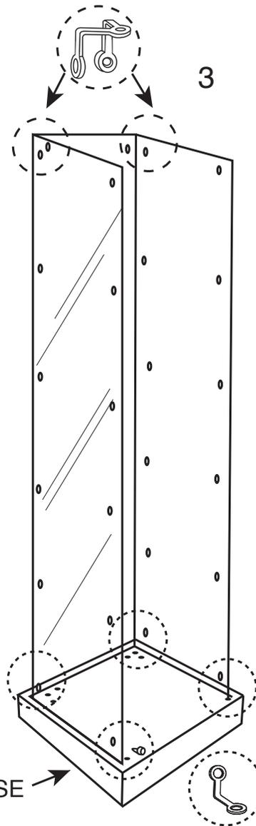
**STEP 5. PLACE TOP GLASS ONTO ASSEMBLY ALONG WITH ALUMINUM STABILIZING BAR ATTACHING ALLEN SCREW AND PLASTIC WASHERS AND L-BRACKETS.**
